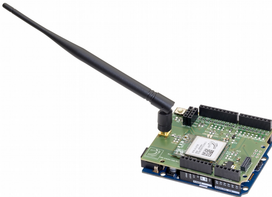
Figure 3. EMB-Arduino-Cape-1272 installation onto the Arduino Zero board.
