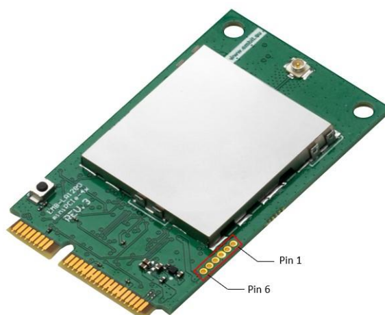
Figure 3: Programming pin configuration
